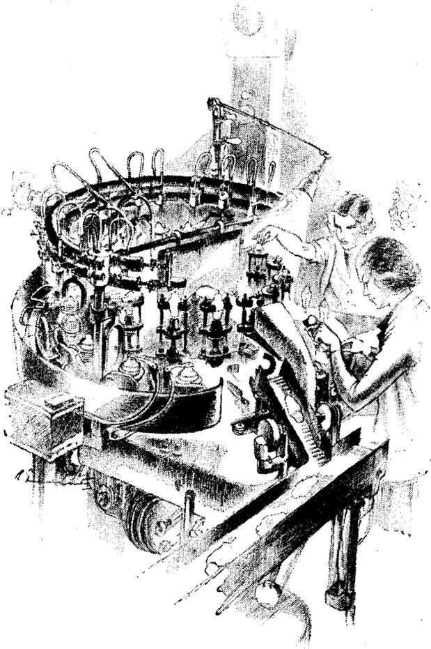
One of the many intricate machines used in the Australian Radiotron Valve Factory for the manufacture of broadcast receiving type valves, is the "Sealex" Machine, illustrated above. Only two manual operations are performed; the machine automatically seals the bulb on the stem, evacuates it, raises the electrodes to incandescence, getters the valves, and finally seals and lifts them on to a moving belt.
