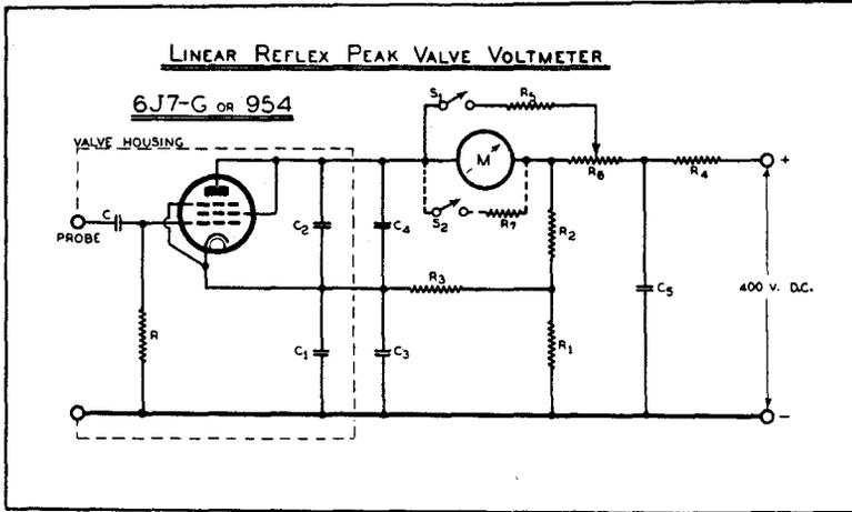
Figure 1. A.C. Operated Linear Reflex Peak Voltmeter.
