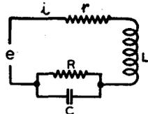
Figure 5. General case of series circuit.
