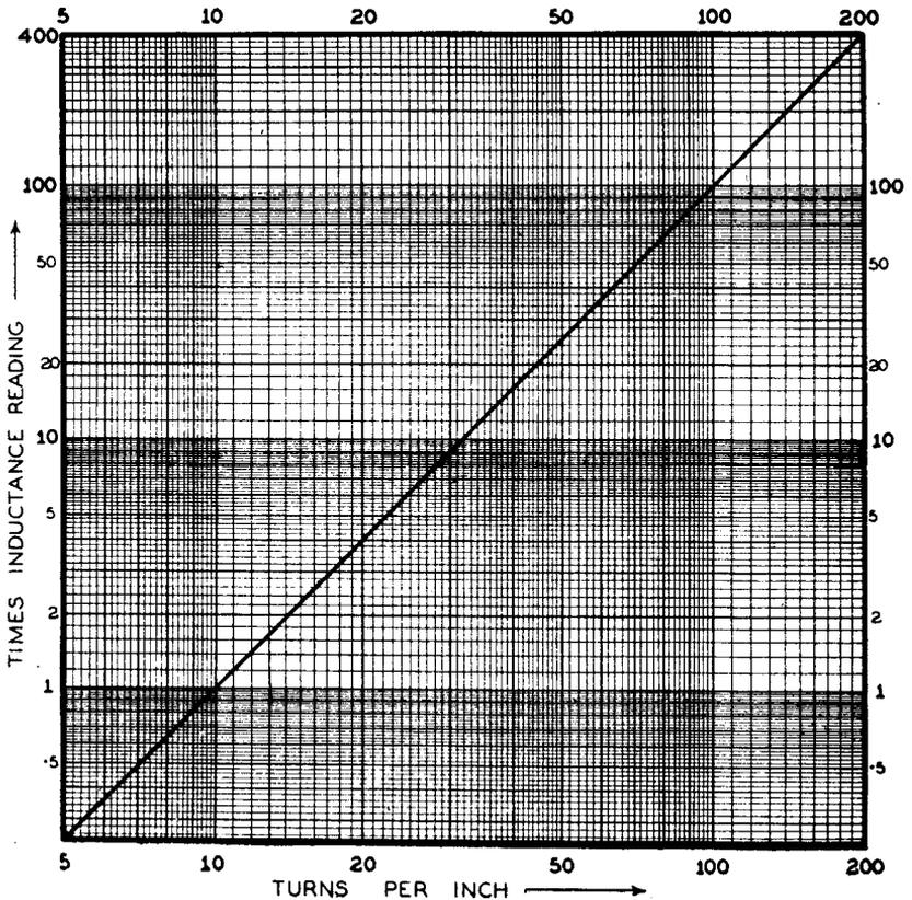
Figure 4: Winding pitch correction for Figure 3.
