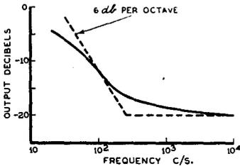
Figure 23 (left). Frequency characteristic (solid line) of Fig. 22 when  $R_1 = 0.225$  megohm;  $R_2 = 25,000$  ohms;  $R_3 = 1.0$  megohm potentiometer; and  $C = 0.02 \mu\text{F}$ . Under these conditions, the bass boost approaches the 6 db. per octave required for complete compensation of recording loss.
