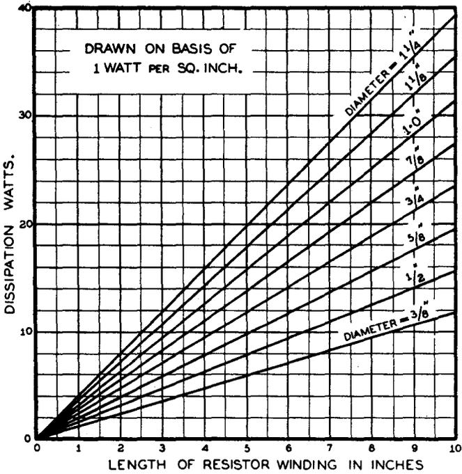
This chart has been drawn on the basis of 1 watt dissipation per square inch of winding. It may be used for other dissipation ratings by multiplying by the appropriate factor. It may also be used for lengths under 1" by dividing both the length and dissipation scale readings by 10.
